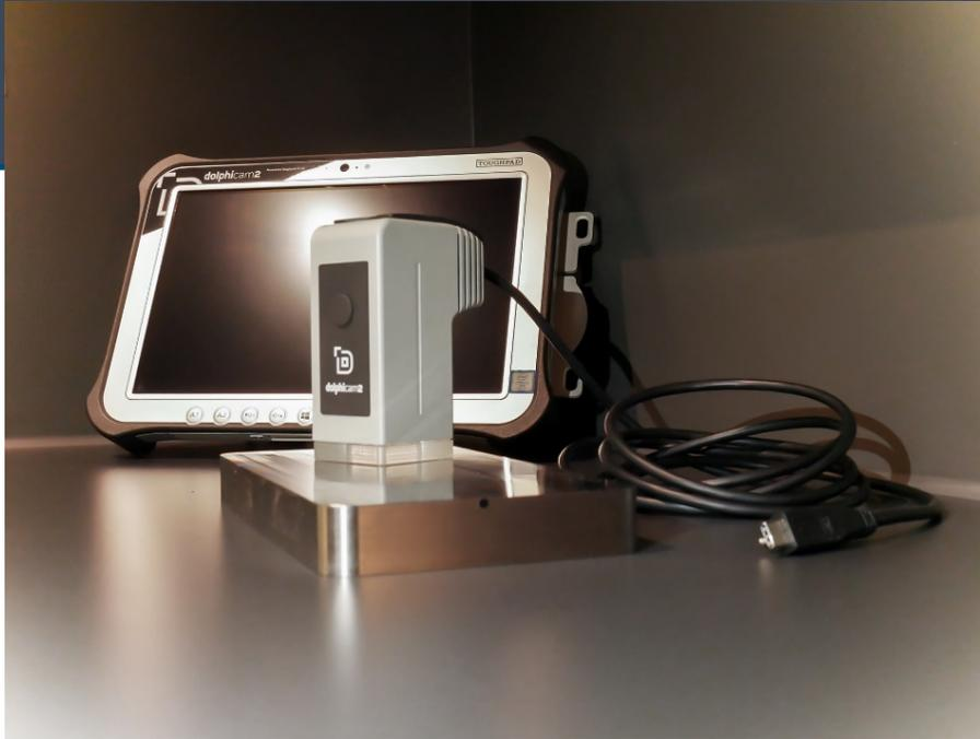
The dolphicam2 is capable of high-resolution imaging and precise measurements for a wide range of material types including composites, metals and multi materials.
